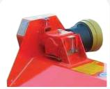
Triple V Belt Drive & Over-Run Gearbox
